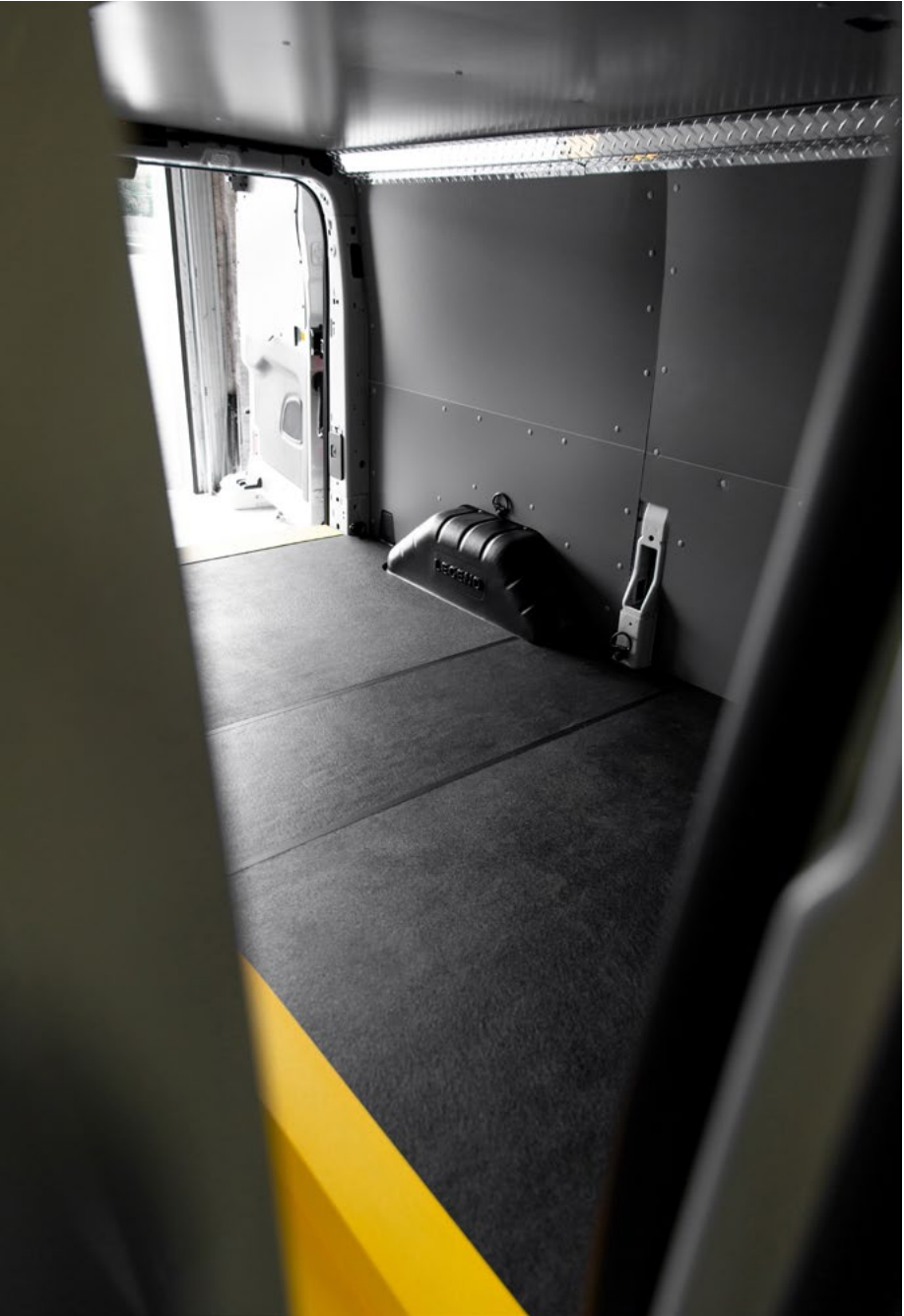
Legend Complete Kit in Transit 130" Low-Roof Van. Shown: StabiliGrip Rigid Floor, Insulated DuraTherm Wall, Ceiling, and Door Liner, Yellow Side and Rear Step Thresholds, Wheel Well Covers.
