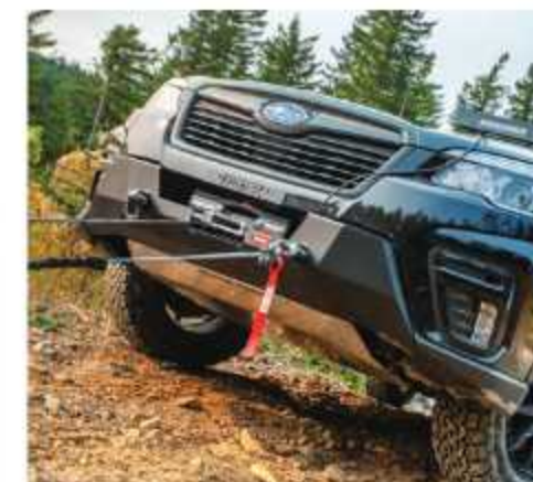
Semi-Hidden Kits for Subaru are compatible with winches up to 6,000 lbs. with mounting pattern of 3.0" x 6.59"
