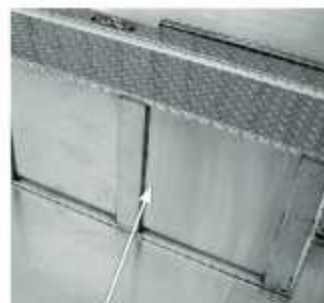
Under body support for added strength
