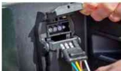
Plugs into USCAR socket to provide 4- and 7-way trailer wiring connectors
