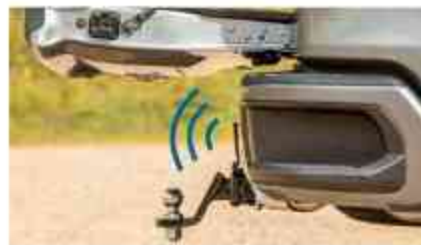
Prevents deployment of inner tailgate panel when ball mount is installed
