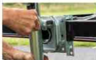
Heavy-duty pull-pin locks jack securely in place
