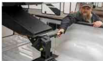
Easy-to-reach release handle for ergonomic locking and unlocking operation of the head from the side of the truck bed
