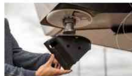
Head piece permanently installs onto kingpin, allowing head channel to guide the kingpin into place for easier hookup
