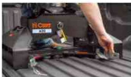
Step 2 - Close the anchor levers to lock the 5th wheel into place
