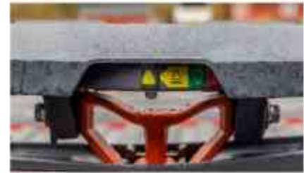
Three-position coupling indicator clearly shows coupling status
