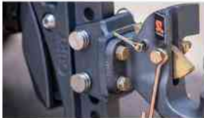
Pintle mount accepts any CURT mount-style pintle hook or ball & pintle hitch (45950)
