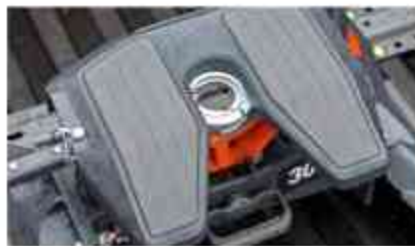
Integrated polyethylene plates for smooth operation, reduced wear and no grease
