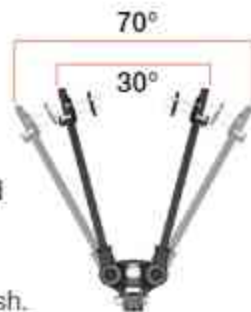
Quick, easy tilt adjustment, no disassembly (excl 17501)
