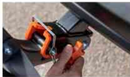
Anti-rattle hitch pin and anti-rattle hand wheel for reduced noise
